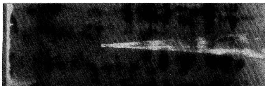
FIGURE 19. China-clay record of vortex structure of a turbulent wake on a flat plate. Cylindrical excrescence, height 0.04 in., diameter 0.2 in. 0.75 ft. from leading edge; wind speed 40 ft./s.
